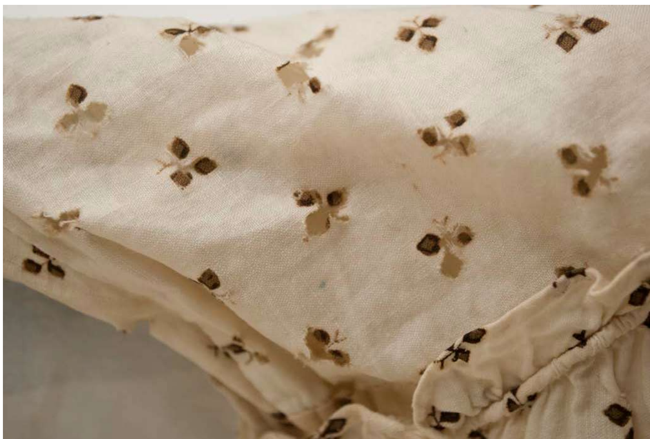
Fig. 1. Printed cotton dress, showing loss of the iron-tannate-printed elements (Courtesy of the Putnam Historical Society, #29 31-A).
