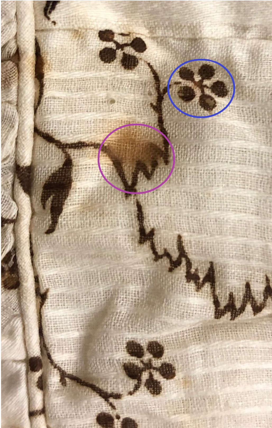
Fig. 3. Examples of loss of mechanical strength (blue circle) and cross-linking (purple circle) caused by iron-tannate dyes (MFIT P87.20.13A).
